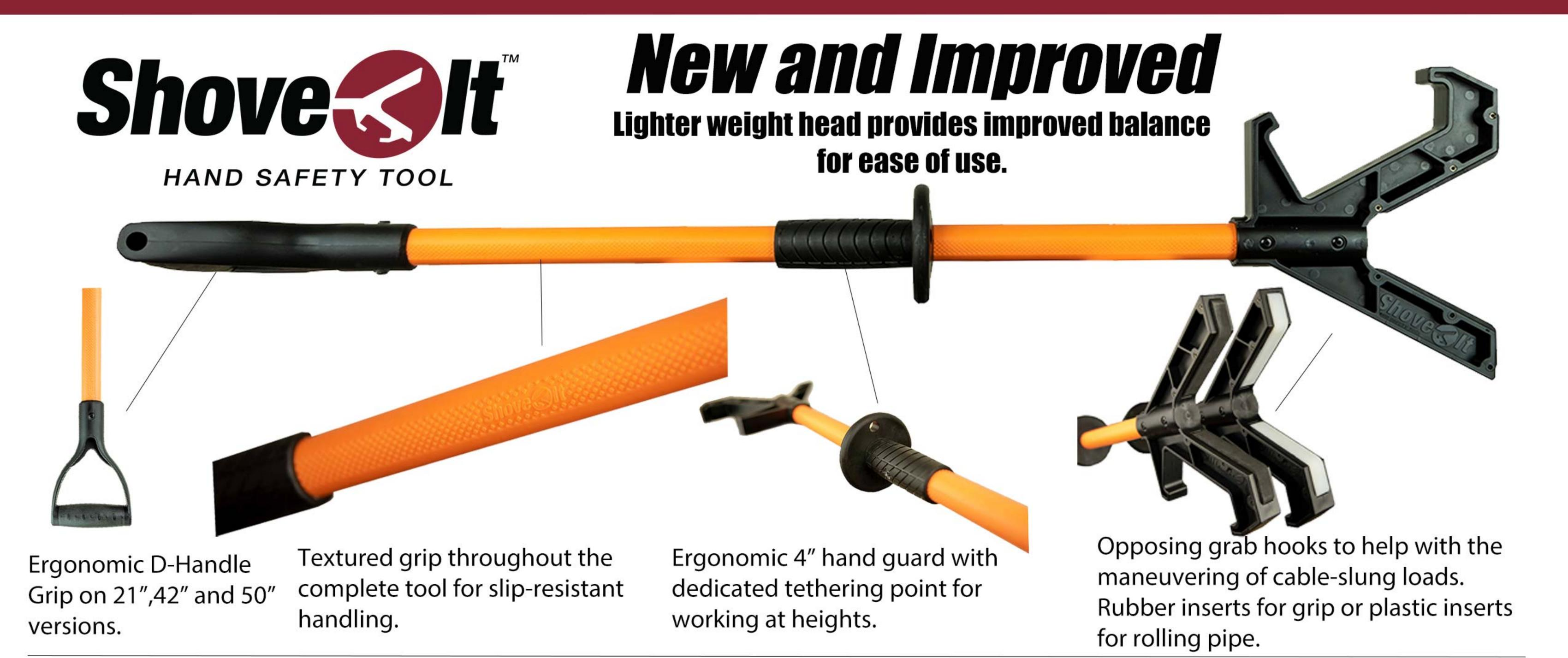
LHR's Shovelt Hand Safety Tool helps avoid hand injuries while working with suspeneded loads. This proprietary Hand Safety Tool helps:
